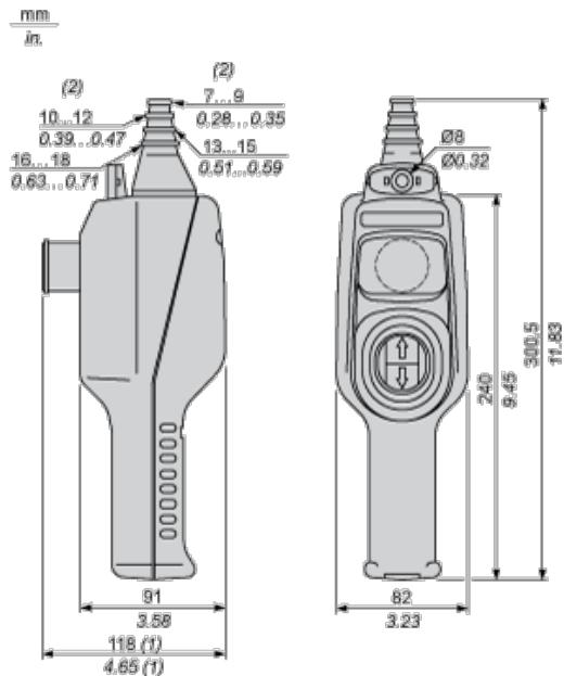
(1) With trigger action latching Ø 30 mm / 1.18 in. Emergency stop.
