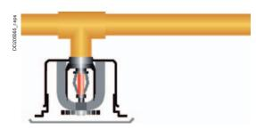
A sprinkler is a sprinkling device blanked off by a heat-sensitive component. It is designed to deliver water when the temperature to which it is subjected exceeds its calibration value.
