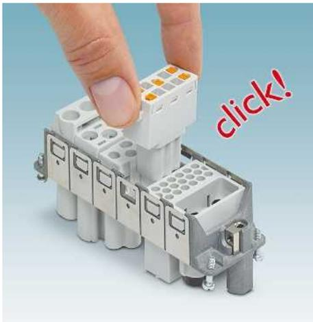
HEAVYCON modular offers space and cost savings by combining several connectors into one. The modular inserts fit in size HC-B housings (HC-EVO, HC-STA, HC-ADV, etc.). Pin and socket modules can be freely combined and are polarized to prevent mismatching.
