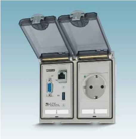
The socket can be operated independently of the control cabinet circuit. In the event of an error, this enables the use of current-operated external measurement devices, which are used for fault analysis. An LED display advises of the voltage connected to the socket.
