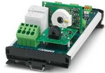
Basic NAR AC charging controller, DIN rail housing, charging case C, level 2
