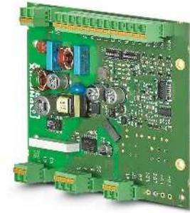
Basic AC charging controller, PCB, charging case C, with MSTB connection
