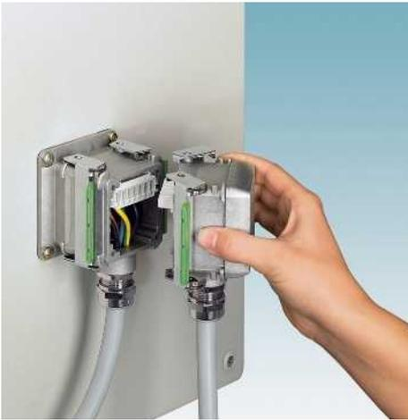
DUPLICON is a consistent power distribution system for 6 x 4 mm<sup>2</sup> and PE conductors (25 A / 400/690 V). Possible applications range from the busbar to ST-COMBI in the control cabinet through to the PCB or plug-in connection on the power consumer. The system has a minimum of components and is flexible in terms of handling. The robust metal housing with vibration-proof locking latches qualifies DUPLICON for the harshest operating conditions.
