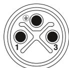
Pin assignment of M12 connector, 2-pos.+PE, S-coded, pin side view
