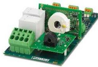
Basic NAR AC charging controller, PCB, charging case C, level 2
