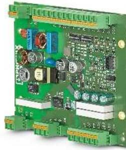
Basic AC charging controller, PCB, charging case B, with MSTB connection
