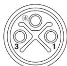
Pin assignment of M12 socket, 2-pos.+PE, S-coded, socket side view
